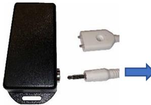
4. When connection OK/Success is displayed, reconnect the sensor cable to the WL module and the connection is completed.
